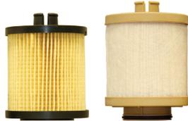
When installed both filters seal radially, however the sealing point is different for each. The OE style filter seats and seals in the ID of the flange in the filter housing. This design requires an extended area at the bottom of the filter which fits into the flange area. The radial seal is formed as the filter is seated.
